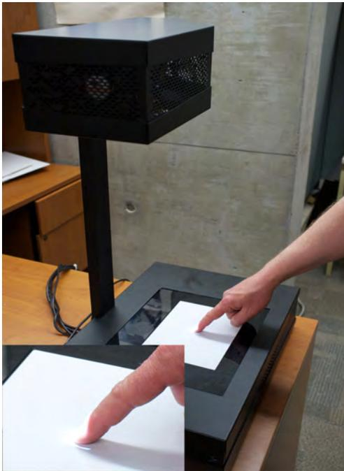
**Figure 5: The FMT demonstrator. Note the dot of light on the finger, emanating from the high-speed projector.**
